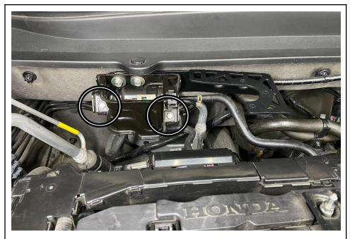
7. Reinstall the fuel hose cover using the factory bolts.
