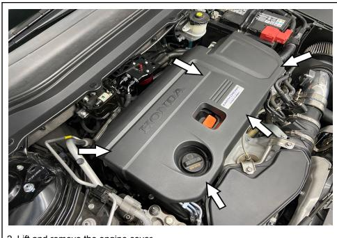
2. Lift and remove the engine cover.
