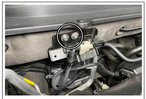
5. Remove the two 10mm bolts securing the fuel line assembly bracket.
