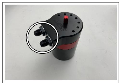
9. Secure the two -6 AN to M16  $\times$  1.5 fittings along with the provided crush washers onto the HPS oil catch can.
