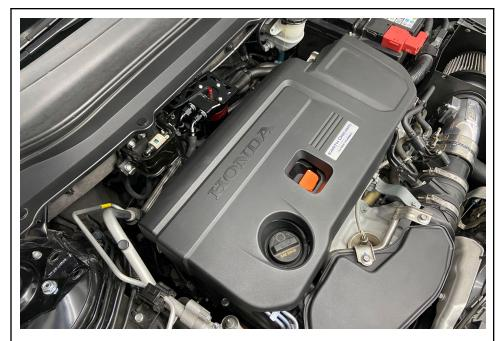
15. Reinstall the engine cover back onto the vehicle.
