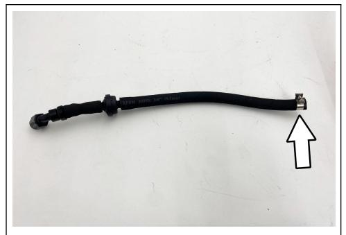
13. Slide the provided FIC-13 clamp onto the hose with the pre-assembled 45 degree fitting.
